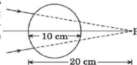
**Q10.** A point 'O' marked on the surface of a glass sphere of diameter 20 cm is viewed through glass from the position directly opposite to the point O. If the refractive index of the glass is 1.5, find the position of the image formed. Also, draw the ray diagram for the formation of the image.
